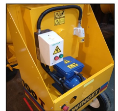
Electric motor drive -110 volt, 1 phase
