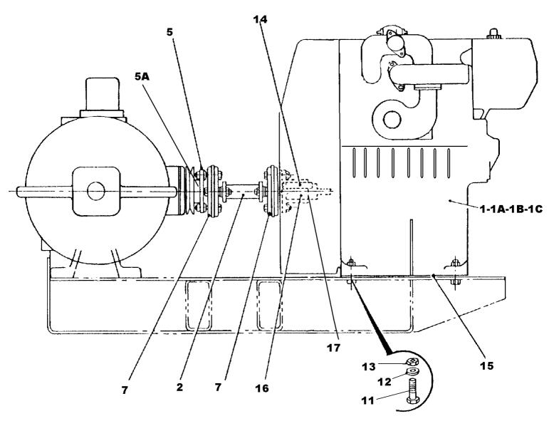
CENTRES OF ENGINE AND GEARBOX OUTPUT/INPUT SHAFTS MUST BE ALIGNED TO AVOID STRAINING SHAFT AND LAYRUB COUPLINGS.
