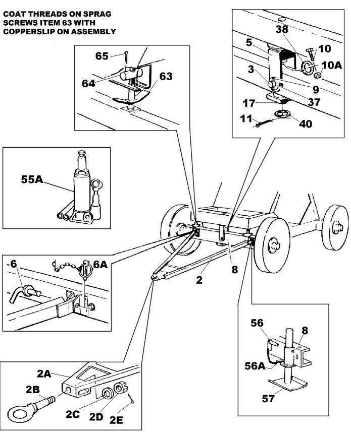
ITEM 2B, NATO TOWING EYE SHOULD BE CROSS DRILLED ON ASSEMBLY TO ENABLE FITMENT OF SPLIT PIN ITEM 2E
