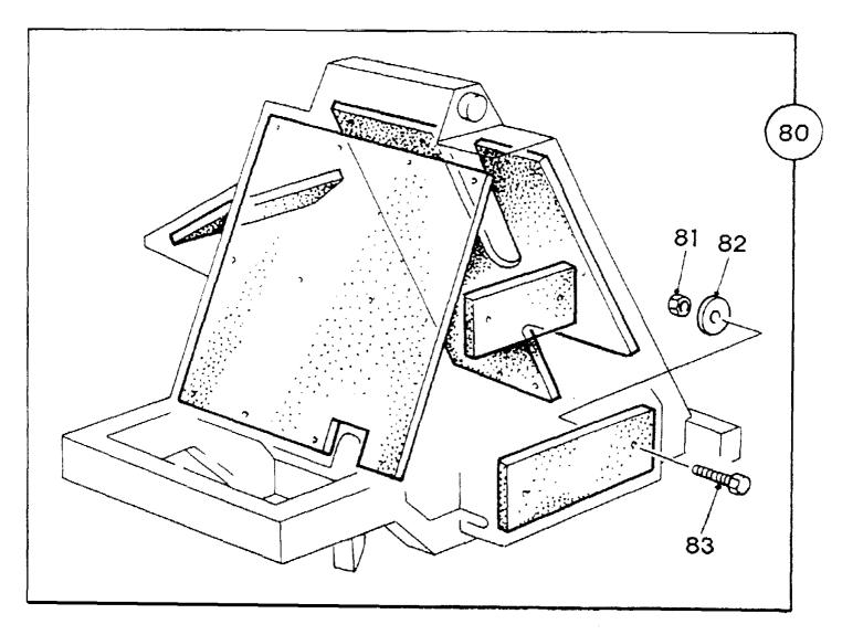
REFER TO THE ENGINEERING DRAWING WHEN DRILLING THE MAINFRAME AND PANELS TO SECURE THE CLADDING KIT.
