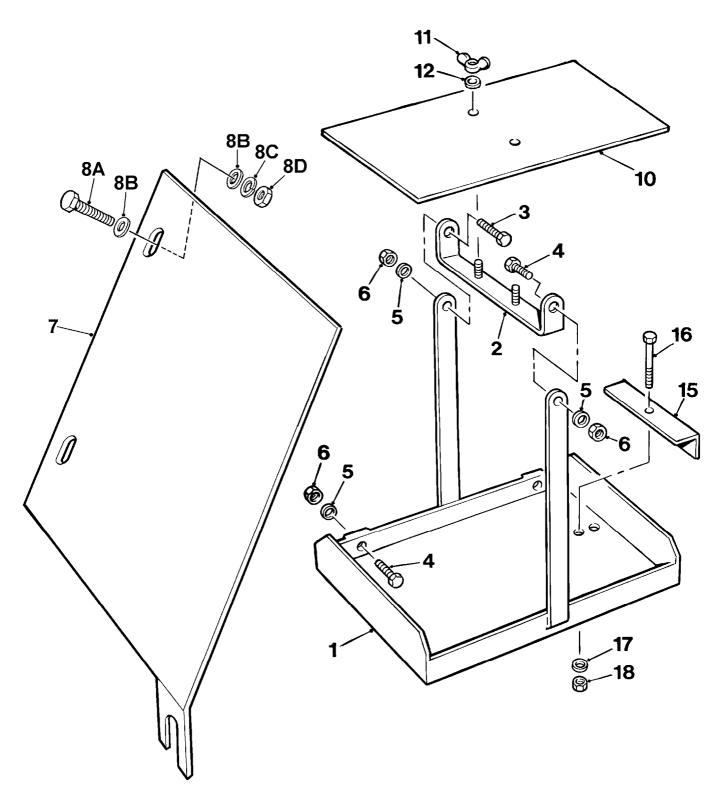
EARLY MACHINES REQUIRE THE MAINFRAME DRILLING TO THE LEFT HAND SIDE OF THE ENGINE BED SO THAT THE BATTERY TRAY CAN BE ATTACHED. THE MAINFRAME OF LATER MACHINES IS PREDRILLED DURING MANUFACTURE.
