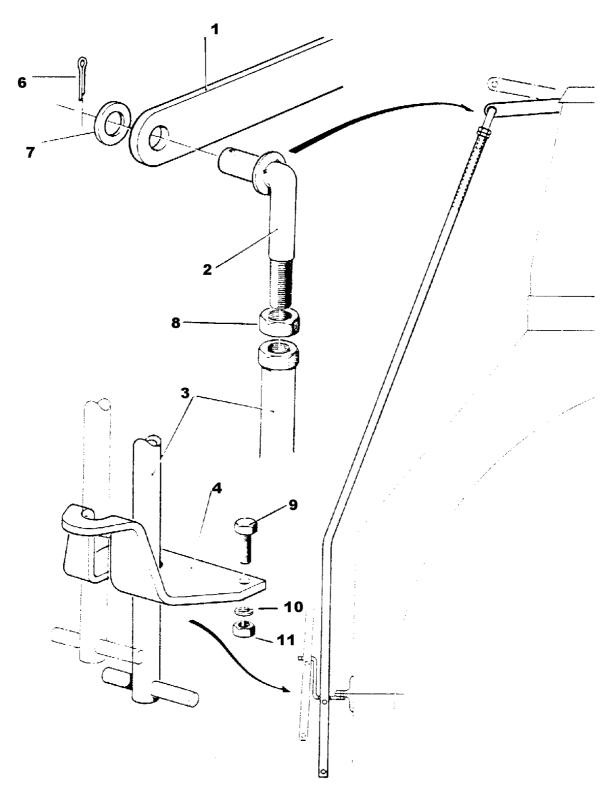
COAT THE THREADS ON ITEM 2 WITH COPPER SLIP ON ASSEMBLY
