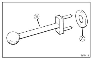
Figure 2.15.1 Valve Spring Compressor
