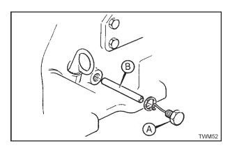
Figure 2.44.3 Centre Bearing Dowel
