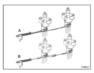
Figure 2.27.1 Fuel Pump Linkage A - Early TS/TR; B - Later TS/TR and all TX
