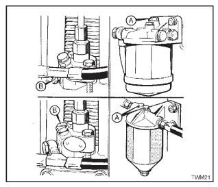
Figure 2.24.1 Priming the Fuel System
