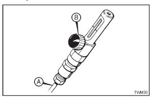
Figure 2.28.3 Fuel Pump Timing Gauge - 317-50518
