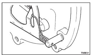
Figure 2.31.2 Variable Speed Return Spring
