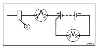
Figure 7.3.1 Test Instrument Connection Diagram X - Removed B+ Battery Terminal
