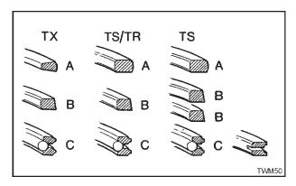
Figure 2.40.1 Piston Rings A - Firing Ring; B - Compression Ring; C - Oil Control Ring
