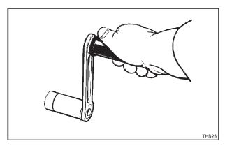
Figure 4.1.2 Holding the Starting Handle
