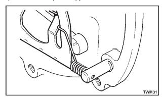
Figure 2.30.1 Variable Speed Return Spring
