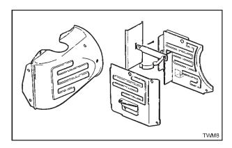
6. Remove the gear end air shield; it may be necessary to slacken the axial fan before the shield can be removed.
