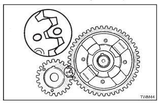
Figure 2.36.1 Gear Timing Marks
