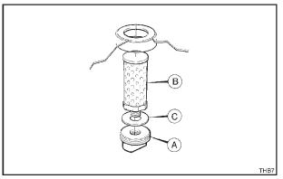
Figure 2.23.1 Fuel Tank Internal Filter
