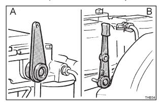
Figure 4.2.3 Decompressor Lever - A - TS/TR; B - TX
