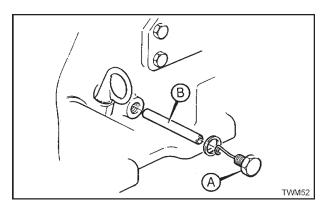
Figure 2.43.1 Centre Bearing Dowel
