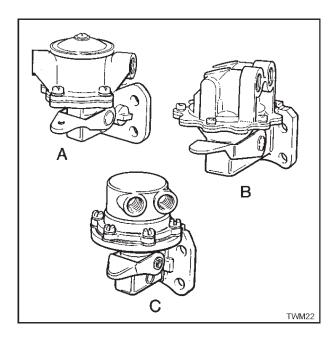
Figure 2.25.1 Fuel Lift Pumps A - AC Delco; B - Pienne; C - Corona
