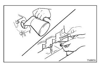
Figure 2.51.1 Oil Filler and Drain
