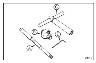
Figure 2.17.1 Recess and Seat Cutting Tool
