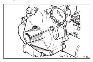
Figure 4.2.3 Starting Handle Housing
