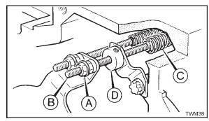
Figure 2.31.6 Excess Fuel Trip - TX
