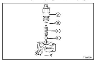
Figure 02.28.1 Fuel Pump Components
