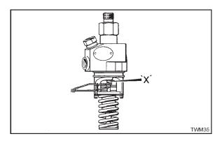
Figure 2.31.5 Fuel Pump Calibration Marks
