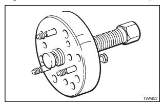
Figure 2.44.1 Crankshaft Gear Removal Tool
