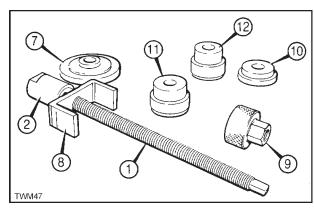
Figure 2.38.1 Camshaft Bush Tool 393235
