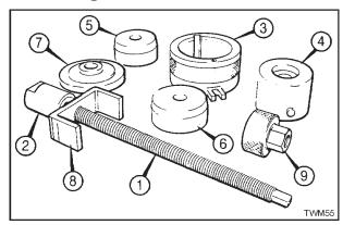
Figure 2.47.1 Main Bearing Tool
