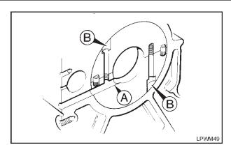
Figure 2.44.4 Dowel Hole Alignment A - Dowel Hole; B - Capscrew Head Recess
