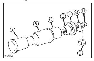
Figure 2.47.2 Main Bearing Tool 317-50006
