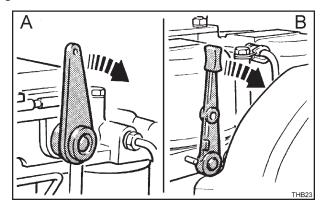
Figure 4.3.1 Decompressor Lever - A - TS/TR; B - TX
