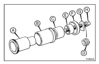
Figure 2.38.2 Camshaft Bush Tool 317-50006
