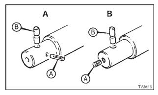
Figure 2.21.1 Starting Handle Pin A - Early Engines; B - Later Engines
