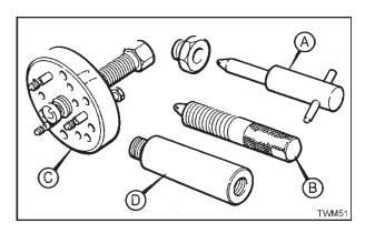
Figure 2.41.1 Flywheel Tools: A - Early Locking Tool; B - Current Locking Tool; C - Puller; D - Mandrel
