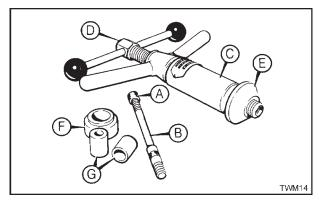
Figure 2.16.1 Valve Guide Tool
