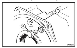
Figure 2.36.2 Camshaft End Float Access
