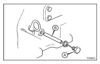
Figure 2.44.2 Centre Bearing Dowel
