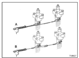
Figure 2.29.1 Fuel Pump Linkage A - Early TS/TR; B - Later TS/TR an all TX
