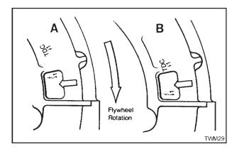
Figure 2.28.2 Flywheel Timing Marks
