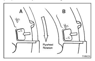
Figure 2.28.3 Flywheel Timing Marks
