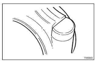
Figure 2.39.1 Bearing Cap Bolt Head Location
