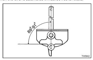
Figure 2.34.2 Speed Control Lever
