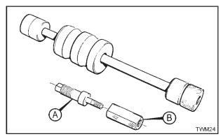
Figure 2.26.2 Injector Removal Tool
