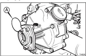
Figure 4.2.4 Starting Handle Housing
