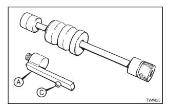
Figure 2.26.1 Injector Removal Tool with Early Type Adaptor
