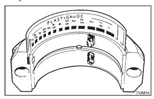
Figure 2.46.1 Checking Bearing Clearance
