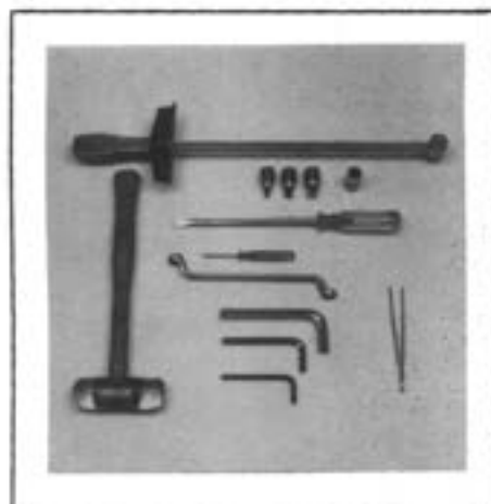
F Torque wrench 0-7 daNm. 13 mm socket spanner. 6, 8 and 12 mm hexagon sockets. 12 mm screwdriver. 2 mm screwdriver. 13 mm ring spanner. 6, 8 and 12 mm hexagon socket spanners. Plastic hammer. Tweezers.
