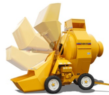
hopper raises hydraulically for drum charging
