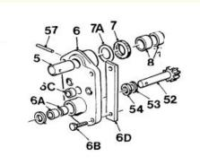
**Tilting Pinion Assembly for Handwheel** Complete castings assembly with pinion, stub pin and all bushes and bearings (fully lubricated).
