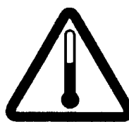
General hot surface warning
