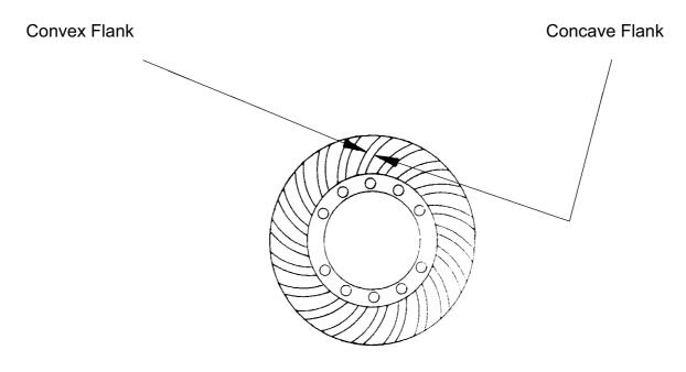
The markings on a crownwheel which is correctly meshed with the pinion should resemble those shown on the illustration below:-
