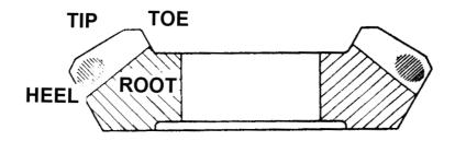
Contact markings closer to heel and tip than factory markings.
