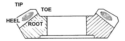
Although the contact point on both flanks of the teeth may vary slightly, generally speaking when correctly setup the markings on both the convex and concave flanks will be in the centre of the tooth form and can still be considered to be correct if, on both flanks, the markings are towards the toe or if crossed slightly e.g. towards the toe on the convex flank and the heel on the concave flank or vice-versa.
