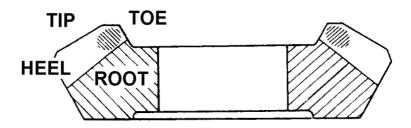
Contact markings closer to toe and tip than factory markings
