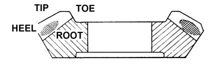
Contact markings closer to heel and root than factory markings
