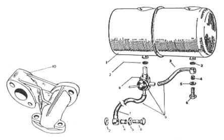
Engines operating on Kerosene are fitted with the following additional and/or alternative parts:-
