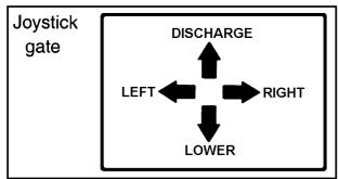
Because of the gate it is not possible to move the lever diagonally, therefore it is not possible to tip and slew the skip simultaneously.
