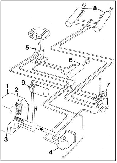
steering wheel is turned. If the oil flow from the pump (4) fails, the steering unit can function as a handpump; this will allow the machine to be steered, but without power assistance.
