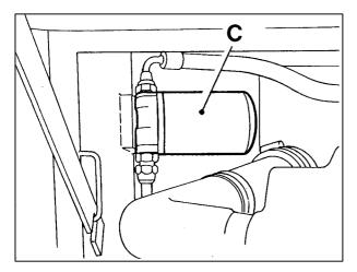
Clean joint area, wipe with hydraulic oil, and fit new cartridge.
