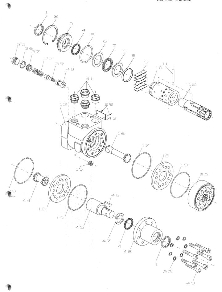
Hydraulic Steering Units HKU, HKUS and Torque Amplifier UVM, Service Manual Dismantling (ref. Item pos. 1÷51 from exploded views, see pages 20÷22)
