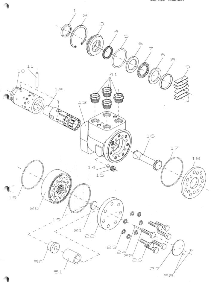
Hydrostatic Steering Unit **HKUS**Metric and SAE versions
