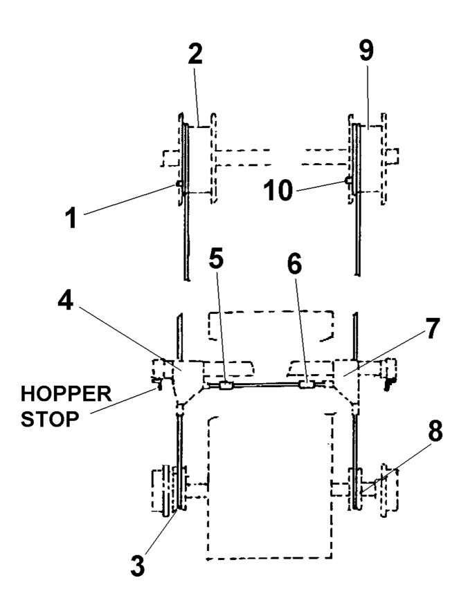
rope retainer blocks, items 5 and 6, located on the section of wire rope between the two rope guides at the back of the bin.
