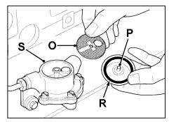
Assemble the lift pump. Use a good joint and ensure that the lift pump body and cover are fitted together correctly because leakage at this point will let air into the fuel system. Fit the heat shield, if one is fitted.
