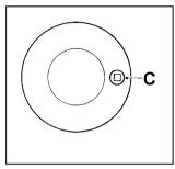
If the oil level is low, top up with clean oil of the correct grade
