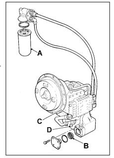
Clean the drain plug (it is fitted with a magnetic insert), and the sealing surface of the housing.
