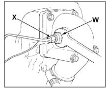
Note: For Lucas fuel injection pumps: Loosen the union nut at the outlet connection of the low pressure fuel leak off pipe which is on top of the governor housing of the fuel injection pump. Operate the priming lever of the fuel lift pump until fuel. free of air comes from the connection. Tighten the union nut.
