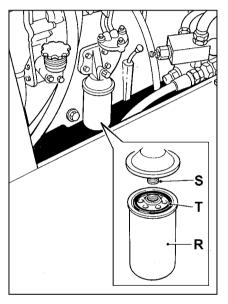
To prevent the engine from starting, disconnect the electrical stop control of the fuel injection pump. Turn the starter key to operate the starter motor until oil pressure is obtained. Oil pressure is indicated when the warning light is extinguished or by a reading on the gauge. Re-connect the electrical stop control of the fuel injection pump.
