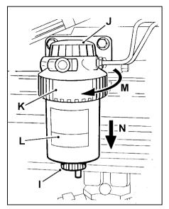
Remove the canister from the filter head by a direct pull downwards (N), and discard the old canister.
