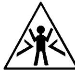
Keep clear of this “Crush area” between the front and rear articulating chassis of the truck.
