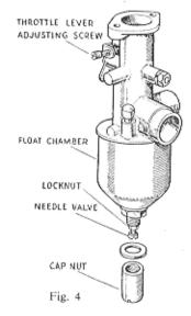
Now test with the engine off load, and adjust the throttle adjusting screw, so that it just bears lightly on the buffer spring. In this condition the engine should run steadily, without "hunting." The locknut on the needle valve should now be tightened.
