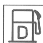
Diesel fuel fill
