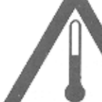
General hot surface warning
